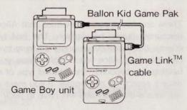
Connect the Game Link<sup>TM</sup> cable as shown in the diagram. After checking that both Game Paks are set properly, turn on the power switch on both units.
